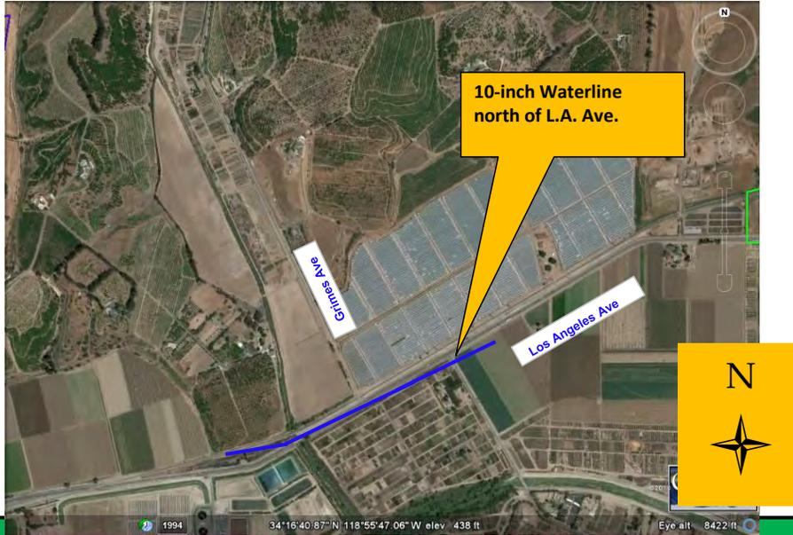
Install approximately 5,000 lf of 10-inch water line and appurtenant work to improve operational flexibility in the system per Master Plan.
